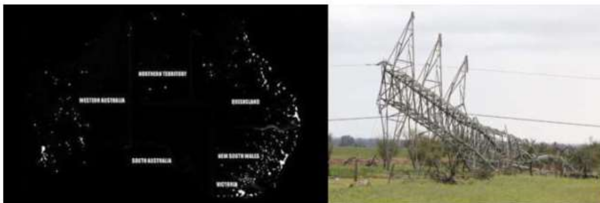
Figure 1. Satellite image of Australia taken on September 28, 2016, shows the blackout across the state of South Australia and the aftermath of the Storm that damaged Transmission Lines which triggered the blackout (RNZ, 2016)
